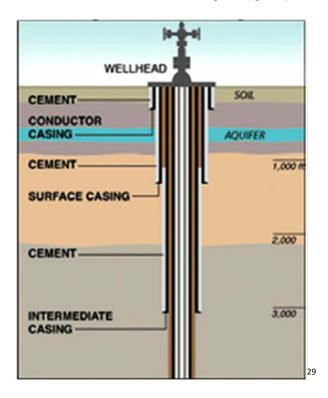
In the process of inserting and cementing pipes through aquifers, the potential exists for cracks to develop, which can allow leaks into the water table. We believe one case of this happening is one too many. Industry officials need to take the lead on promoting best practices as they may understand safety better than the regulating bodies.
